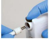
2. Disconnect the Helmet Power Cord from the Battery - Press down on the Secure Lock (Black) Button to release, then pull the cord connector out from the Battery connection receptacle.
