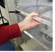
With the Shelf at the desired height, move the Shelf backward to engage the Pins into the Slots.
