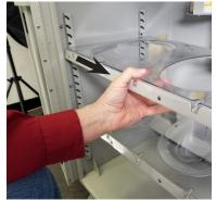
3. Continue to move the Shelf backward and then downward until the Shelf Pins are fully secured in the furthest back and down Slot positions.
