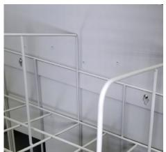
2. Slide the Rack Mounting Slots over the Mounting Screw heads and then down onto the Screw threads.
