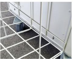
3. Slide the Rack Mounting Slots over the Mounting Screw heads and then down onto the Screw threads.
