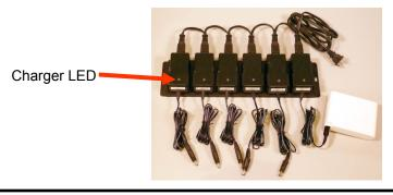
C. Connect from 1 to 6 MAXAIR Li-lon 2000-36/2000-30 batteries to the charger. If the battery needs charging the Charger LED will turn red. It will turn green again when the battery is ready for use. If it remains green, the battery is ready for use.
