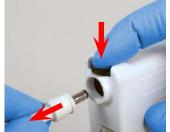
00. Disconnect the Helmet Power Cord from the Battery - Press down on the Secure Lock (Black) Button to release, then pull the cord connector out from the Battery connection receptacle.
