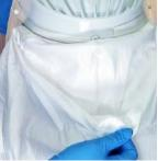
Grasp the back of the Hood Filter and begin to pull the Hood up and over the Helmet.
