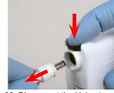
00. Disconnect the Helmet Power Cord from the Battery - Press down on the Secure Lock (Black) Button to release, then pull the cord connector out from the Battery connection receptacle.
