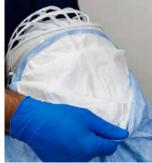
5. Grasp the back of the Hood Filter and begin to pull the Hood up and over the Helmet.
