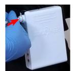
2. Connect Helmet Power Cord to Battery; push Power Cord Connector into the Battery Receptacle until the Secure Connection audibly clicks.
