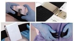
Assemble Battery onto Belt - Place top edge of Belt under the Battery Clip, up to Clip top, so the Clip Detent rests on the Clip Base and NOT the Belt, then place belt around waist with battery near side-back of right hip.
