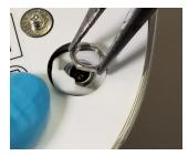
4. Turn Hex Nut until it is loosened away from the Power Jack and remove completely from the connection.
