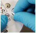
5. Grasp the old TurnLock connector with fingers. If old connector is broken it may be necessary to grasp it with the Needle-nose liers.
