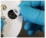
Lift the old TurnLock connector off its mounting on the Power Jack and discard appropriately as potentially contaminated waste.
