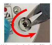
3. Using a standard pair of Needlenose pliers, grasp opposite flat sides of the Hex Nut and loosen by turning coulterclockwise.
