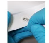
2. From inside the HH, pinch the legs of the Side Turn Clip together with the MAXAIR Screwdriver flat blade, and push the turn Clip out of the HH Skirt.
