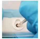
2. Push the Front Vent Clip fully out of the Front Lens Mount.
