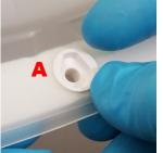
2. Position the Front Lens Mount as shown at A.
