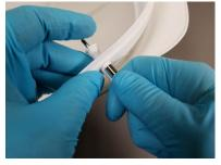
5. Bracing the the HH from the inside, push the screwdriver inward with controlled force to push the Side Turn Clip Base out of the HH.
