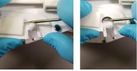
Alternative to step 2, position both thumbs at bottom edge of HH Skirt for support, and use the screwdriver flat blade on top of the protruding post and press down to remove the Lens Mount.
