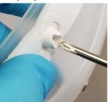
3. From outside the HH, insert the Phillip blade through the Front Lens Mount.
