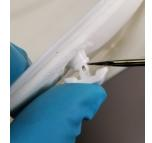
3. From outside the HH, use the screwdriver flat plat to aid in positioning the legs of a Side Turn Clip into the front opening of the Side turn Clip Base.
