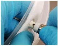
4. Bracing the front of the HH from the inside, push the scredriver inward with controlled force to push the Front Lens Mount out of the HH.
