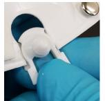
1. Grasp a Side Lens Mount between thumb and forefinger and slide it into the Lens Mount slot in the HH.
