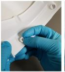
1. From inside the HH, place a new Side Turn Clip Base into the round side hole on the HH.
