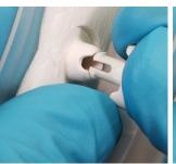
3. From outside the HH, position the legs of a Front Vent Clip into the front opening of the Front Lens Mount.
