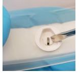
1. From inside the HH, pinch the legs of the Front Vent Clip together with the MAXAIR Screwdriver flat blade.
