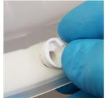
1. From inside the HH, place a new Front Lens Mount into the front hole on the HH.
