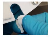
Grasp the Side Lens Mount between thumb and forefinger and pull down and away from the FCC.
