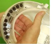
2. Grasp the front of the Liner along the top of the front Headband with the fingers.
