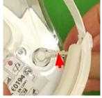
1. Ensure the Power Cord is aligned with the Liner Cord cutout.
