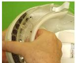
3. With thumb against bottom front of Helmer, pull fingers down and push thumb up to disengage Front Snaps.
