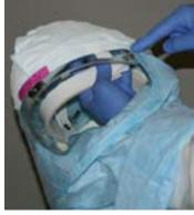
Snap both sides of the Hood to the Helmet by pressing the Hood snaps together with the Helmet side snaps.
