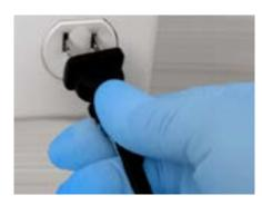
Connect the Charger (single and/or 6-Gang) to an appropriate grounded wall mains power source (120-240 VAC, 50-60 Hz) before connecting to the Battery(ies). The Charger green status LED should turn on.
