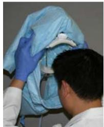
Flip the back side of the Filter Hood up and over the Helmet to the front. Grasp the Helmet on each side with the Filter Hood Lens facing the floor and the Rotary Adjustment Knob facing the ceiling.
