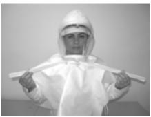
5. Wrap the ties around each other twice to prevent the ties from loosening. There should be a maximum gap distance of approximately 1/4" between the neck and Filter Hood.
