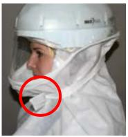
5. There should be a maximum gap distance of approximately 1/4" between the neck and Hood. The user should be able to feel positive pressure airflow across the restricted neck area when the ties are adjusted correctly. The ties should draw the Hood under the chin. If desired, tuck the Hood shroud into the outer body gown for added protection.
