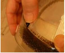
4. Place new rivets into each of the locations where the four were removed in step 1. Place the tip of the rivet in the hole and press down on the rivet head firmly until the rivet is firmly seated in the hole.
