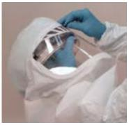
3. Pull the Filter Hood over the front end of the Helmet.
