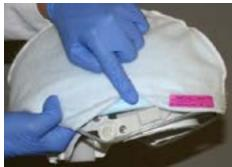
Secure the Velcro pads on each side of the Filter to the respective Velcro strips on the sides of the Helmet by pressing them together.
