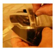
2. Using a thin, flat blade (small screwdriver etc.) pry each rivet up and out of the Cage.
