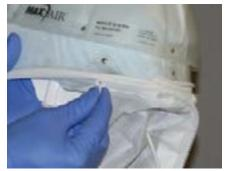
2. Align the zipper on the Cuff, or Shroud, with the mating zipper on the Filter Cover Lens and zip the Cuff or Shroud to the Lens.
