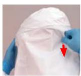
Continuing process of 14, pull Hood all the way down so that Hood Filter (top) is fully down on Helmet.
