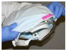
Pull the front of the Filter down over the front of the Helmet, pulling the Filter alignment hole over the center Helmet alignment post of the Helmet.
