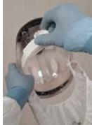
4. Turn Headband Ratchet Knob counterclockwise to loosen headband for ease of donning Helmet.
