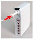
9. Connect the Helmet Power Cord to the Battery. Push the Power Cord Connector into the Battery Receptacle until the Secure Connection audibly clicks.
