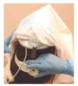
13. Secure Helmet by tightening Ratchet Knob as tight as comfortably possible, while ensuring stability.
