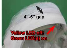
4b. As soon as the Yellow LED turns on - in less than five seconds - open the Bouffant Cap approximately 4" to 5" (10cm to 12cm). Notice the Yellow LED turns off. Close the gap of Bouffant Cap.
