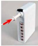
2. Connect the Helmet Power Cord to the Battery. Push the Power Cord Connector into the Battery Receptacle until the Secure Connection audibly clicks.
