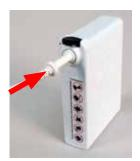
3. Connect the Battery to the Belt and place the Belt around the waist, typically with the Battery towards the rear of the right hip. To begin air flow, insert the Helmet Power Cord Connector into Battery Connector receptacle until the Secure Lock audibly clicks.
