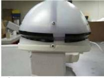
Cut the tape so that it stops in the front-center of the Helmet. This leaves about a one inch open gap.
