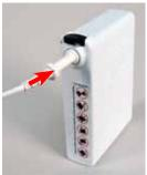
9. Connect the Helmet Power Cord to the Battery. Push the Power Cord Connector into the Battery Receptacle until the Secure Connection audibly clicks.
