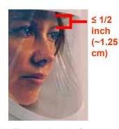
16. Ensure that the front Headband is within 1/2 inch of eyebrows for good visualization of the Safety LEDs
