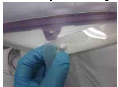
1. Grasp one side DLC flapper and lift away from the Side Attachment Post.
