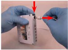
3. Disconnect the Helmet Power Cord from the Battery - push the Secure Connection Button down, pull Cord Connector out, release the Button.
