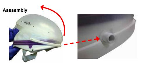
1. Hold the Helmet/Liner/ Filter Cartridge upright by its rear underside with one hand and align/insert the front FCC hole to the Helmet Front Adapter Post. Pull the FCC over and down the back of the Helmet.
