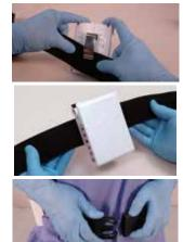
2. Assemble the Battery onto the Belt. Place the top edge of the Belt under the Battery Clip. Move the Belt fully under and up to the top of the Clip. Place the belt comfortably around the waist with the battery near the sideback of the right hip.
