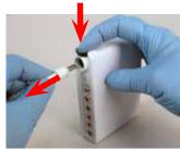
3. Disconnect the Helmet Power Cord from the Battery - push the Secure Connection Button down, pull Cord Connector out, release the Button.
