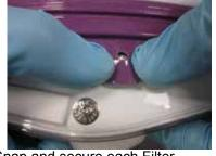
6. Snap and secure each Filter Cartridge side snap tab on to each respective Helmet side upper snap.
