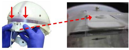
3. With two hands, slide the rear FCC downward so that the FCC T-Tab snaps over the Helmet Rear Adapter Post.
