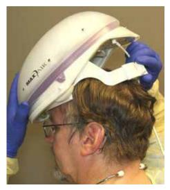
3. Hold the front top of the Helmet in one hand and with the other hand on the Adjustment Knob; lift the Helmet up and off the head.
