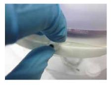
3. Grasp the center of the DLC and lift away from the Helmet. Dispose of the DLC according to your institution's protocol for contaminated waste.
