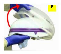
2. Continue pulling up with one hand (E) while pulling down the Helmet and Headband Side Strap with the other hand in the opposite direction (E), until the FCC is up and off the helmet (F).
