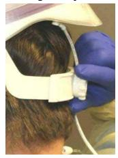
1. Loosen the rear Headband Adjustment Knob (turn counterclockwise).
