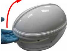
2. Unhook and remove the Helmet Protector lifting from the front and moving upward and off, towards the rear.
