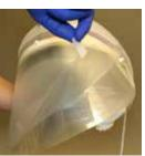
5. Connect the Helmet Power Cord to the Battery. Push the Power Cord Connector into the Battery Receptacle until the Secure Connection audibly clicks.
