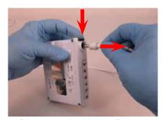
4. Disconnect the Helmet Power Cord from the Battery - push the Secure Connection Button down, pull Cord Connector out, release the Button.
