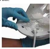
4. Push the rear edge of the Liner inward with your thumb inward. Align the rear Liner holes over the Helmet rear snaps.
