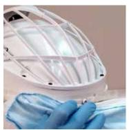
7. Attach center Hood-Lens alignment hole over Helmet center alignment post.
