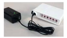
1. Obtain a fully charged battery. (Charger LED should be green after battery is connected to charger for more than 10 seconds.)
