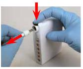
8. Disconnect the Helmet Power Cord from the Battery - push the Secure Connection Button down, pull Cord Connector out, release the Button.
